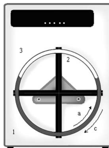
Fig. 1 Schematic diagram of modified Tepe loop system: (1) modified roller pump to obtain a passive blood flow inside the grafts; (2) cross bearing to lodge the grafts closed to a loop; (3) PEtU-PDMS grafts or reference materials partially filled with anticoagulated blood; (a) anticlockwise = direction of graft rotation; (c) clockwise = direction of blood flow into the grafts
